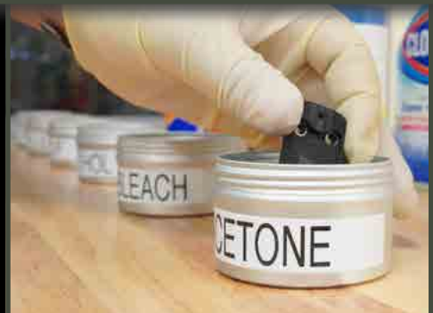
Determines Material Limitations from Contact with Harsh and Common Chemicals
