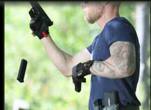
Repeated Drop Testing from Upwards of Two to Six Feet onto Different Surface Mediums
