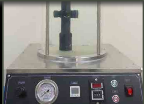
Water and Dust Proof Testing to Ingress Protection (IP) Standards
